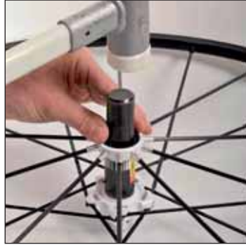
Fit the new bearings using bearing kit 323 909 01.
