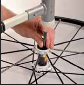
Use the bearing kit to extract the bearings 323 909 01.
